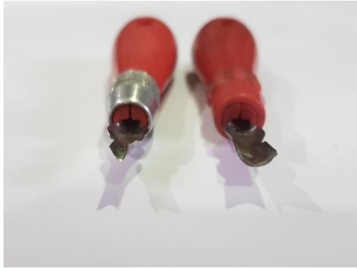
A V-shaped tool (left) & U-shaped tool (right)
